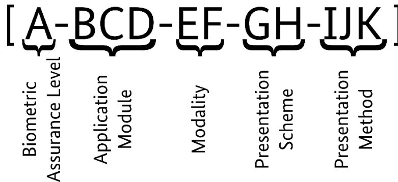
Fig. 4 Generation scheme for an evaluation code. The first curled bracket indicates the target Biometric Assurance Level (“normal” N, “substantial” S and “high” H). The second bracket defines the application module which defines, if necessary, further requirements in addition to the general ones. The third bracket defines the biometric modality used within the application. The presentation scheme used within the modality is indicated by the fourth curled bracket. With the last curled bracket the presentation method shall be declared.
