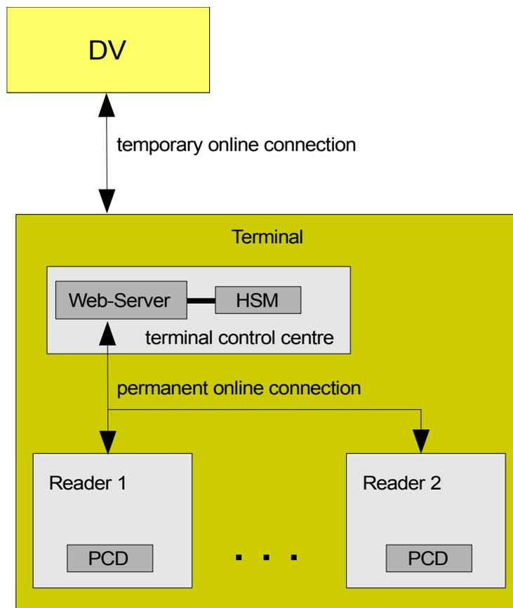
Figure 2: Distributed terminal with local control centre
