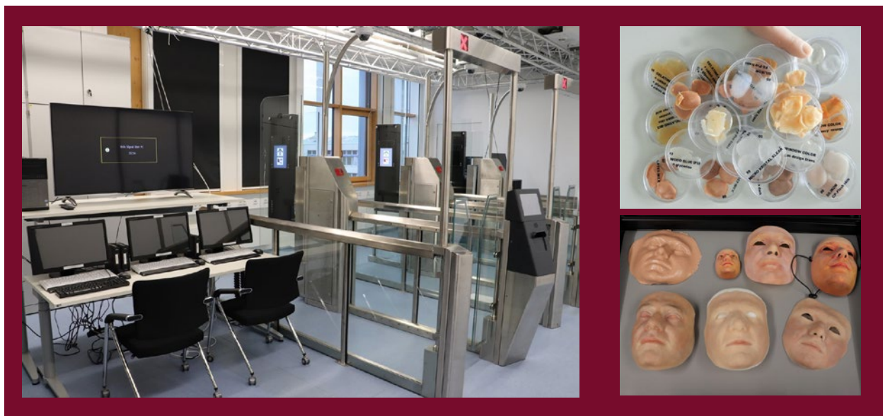
Figure 14: (l) Test facility for the evaluation of national border control systems, as used for parts of the Frontex training courses. By using the EasyPass systems, participants could first observe normal operation of the gates (as used in German border controls) and then attempt attacks aimed at bypassing the systems using forged biometrics. (r) Examples of test equipment used for the vulnerability analysis of face and finger biometrics systems, as utilised in the Frontex training courses.
