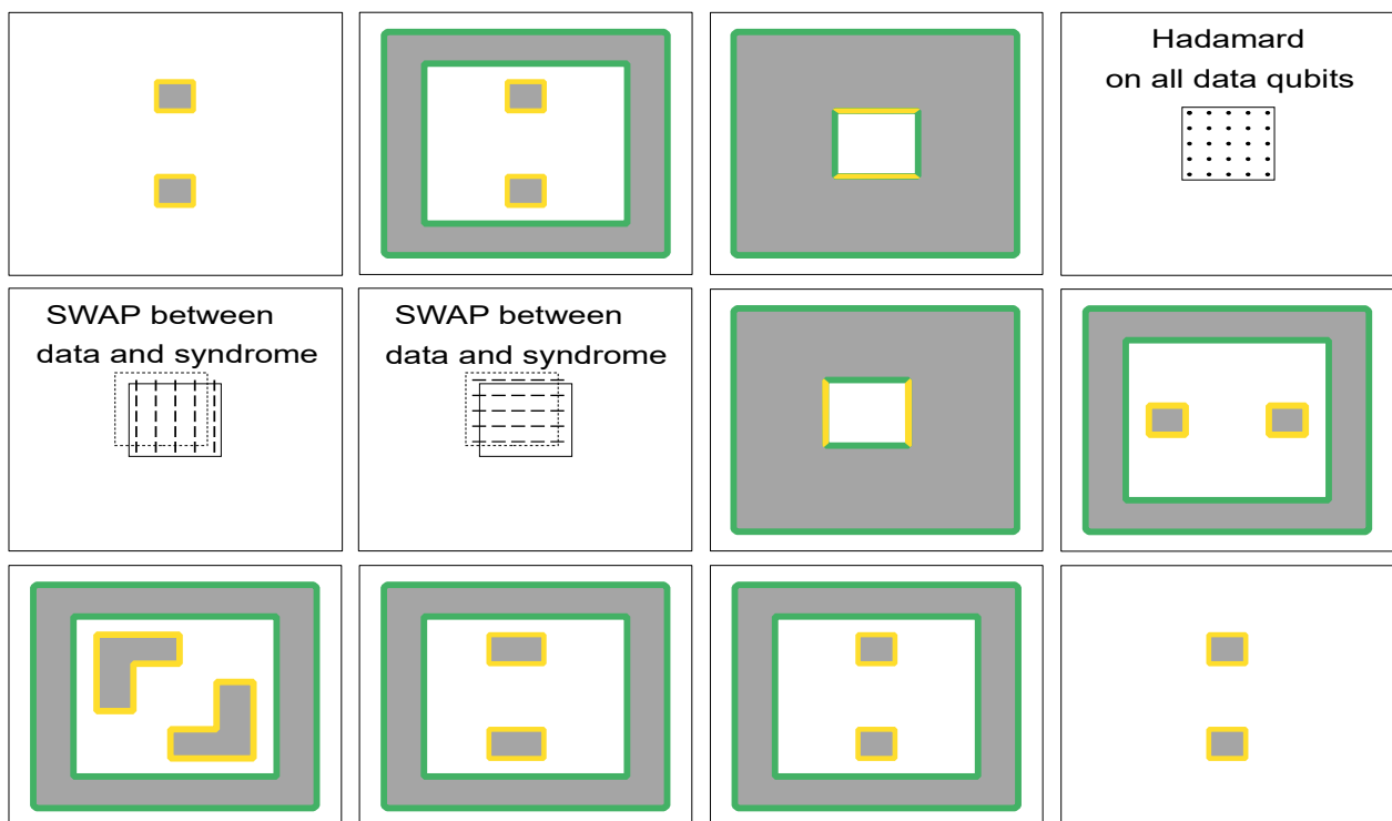
Figure 25.4: Sequence of different stabilizer measurement patterns for a logical Hadamard. Uncolored pictures represent additional physical gates between the stabilizer measurements (number of qubits chosen arbitrary). Here, the physical Hadamards in step 4 can be done during the measurement of the stabilizer cycle before, the physical SWAP gates (step 5–6) can be performed while stabilizer measurements are running in the rest of the array. This sequence basically shows a transformation to a different qubit encoding (step 3), where the logical X and Z operators are just vertical and horizontal lines, on which a Hadamard can be performed easily (steps 4–6) and a transformation back to the original shape of the qubit.
