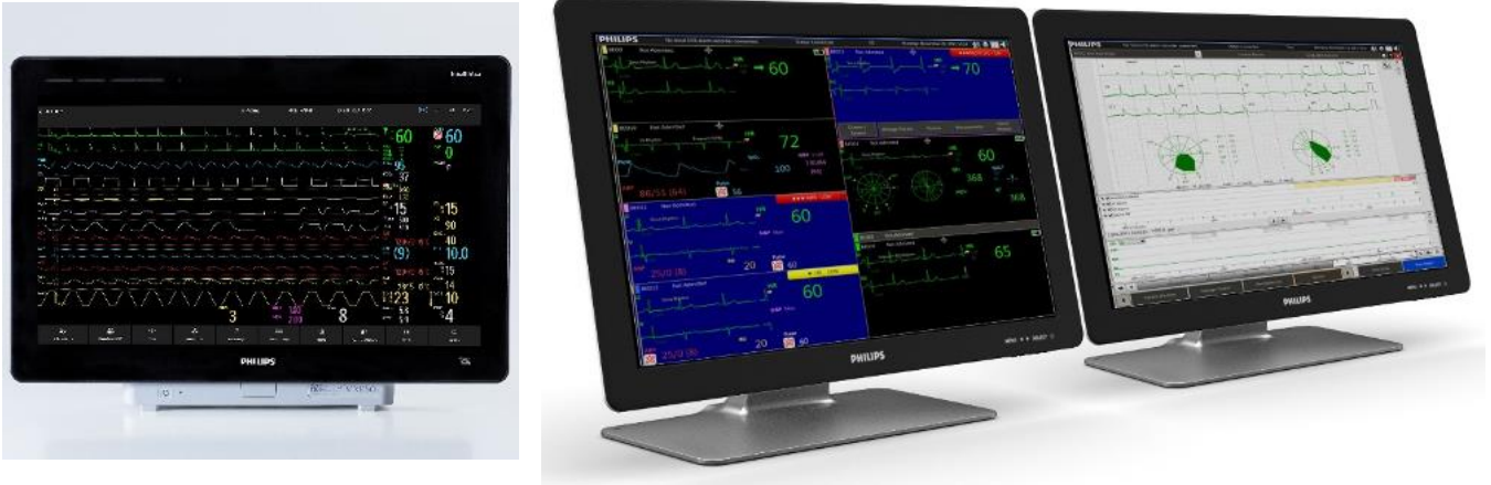
Figure 15: A Philips IntelliVue MX850 patient monitor (left) and PIC iX Surveillance Station (middle + right). (Source: Philips)
