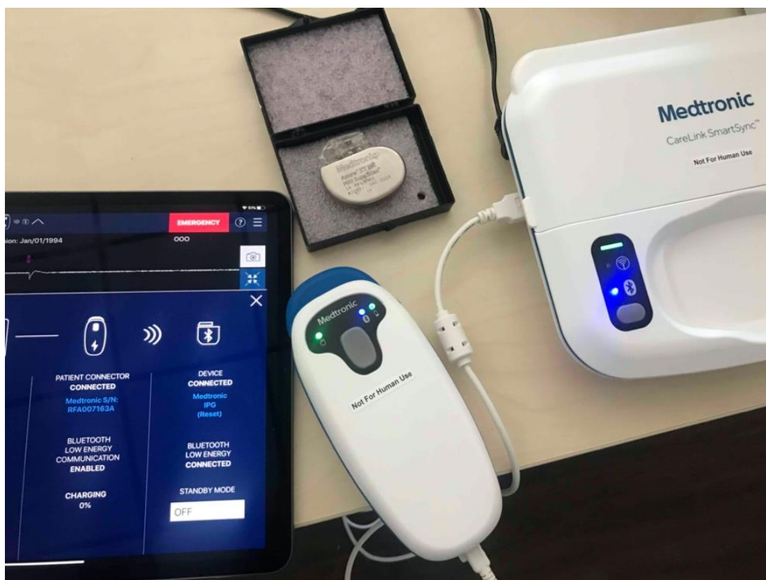
Figure 11: The testing lab of the Medtronic CareLink SmartSync Device Manager system comprising of the base unit (right), a handheld (bottom center) and an iPad with the app (left) as well as a pacemaker (top center). (Source: BSI)
