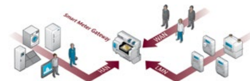
The smart meter gateway as the communication unit in a smart metering system and as the central component between a wide area network (WAN), local metrological network (LMN) and home area network (HAN)
